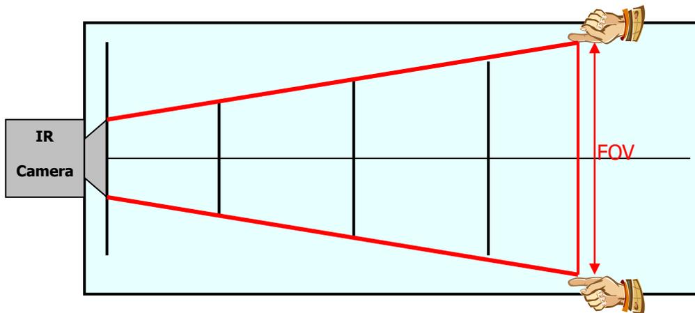
Most thermographers measure a point at 18 inches and then join the points together at the increments marked on the paper and then keep a chart with their camera for easy reference.
