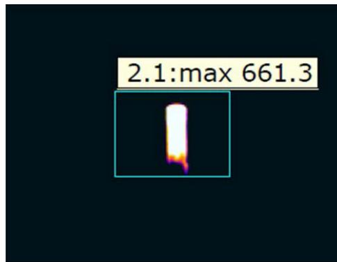
Thermogram 2.2 shows the same target through the Polymer Control Window, with the  $\tau$  set to 0.49 per the baseline established when it was new. The target temperature is shown to be 658.1°F (347.8°C): a 0.49% error between apparent and true temperatures. Again this margin of error is not significant since it is well within the camera's +/- 2% accuracy specifications.
