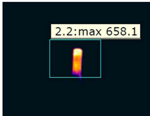
Thermogram 2.3 shows the same target through the CaF2 Test Window, with the  $\tau$  set to 0.49 per the baseline established when it was new. However, in this case the apparent temperature registers as 485.7°F (252.1°C), resulting in a 175.6°F (97.5°C) or 26.55% error between apparent and true temperatures.
