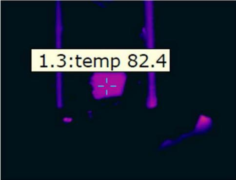
Thermogram 1.4 shows the target after recalibration of the imager to the degraded  $\tau$  value of the CaF2 Test Window. Transmittance was adjusted to 15% to bring the apparent temperature in line with the true temperature. This represents a 69.4% degradation in transmission of the CaF2 Test Window over a two (2) year period.
