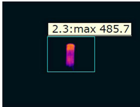
Thermogram 2.4 shows the target after recalibration of the imager to the degraded  $\tau$  value of the CaF<sub>2</sub> Test Window. Transmittance was adjusted to 30% to bring the apparent temperature in line with the known true temperature. Notice that this differs from the 15% transmittance at the lower temperature, confirming Dr. Madding's findings with regard to the variability of Calcium Fluoride's transmittance across the long wave infrared spectrum.
