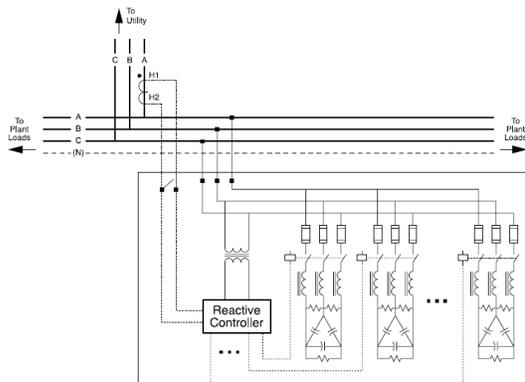
Figure 3: Detuned PFC System Three Line Diagram
