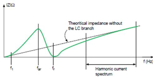
Figure 2: Tuning Point of the Detuned PFC System Branches is  $f_r$  – Below the Harmonics Generated by the Non-linear Loads on the System
