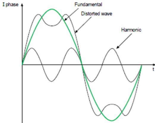
Figure 1: Harmonics are a Mathematical Representation of Distorted Waveforms breaking them down into Component Parts
