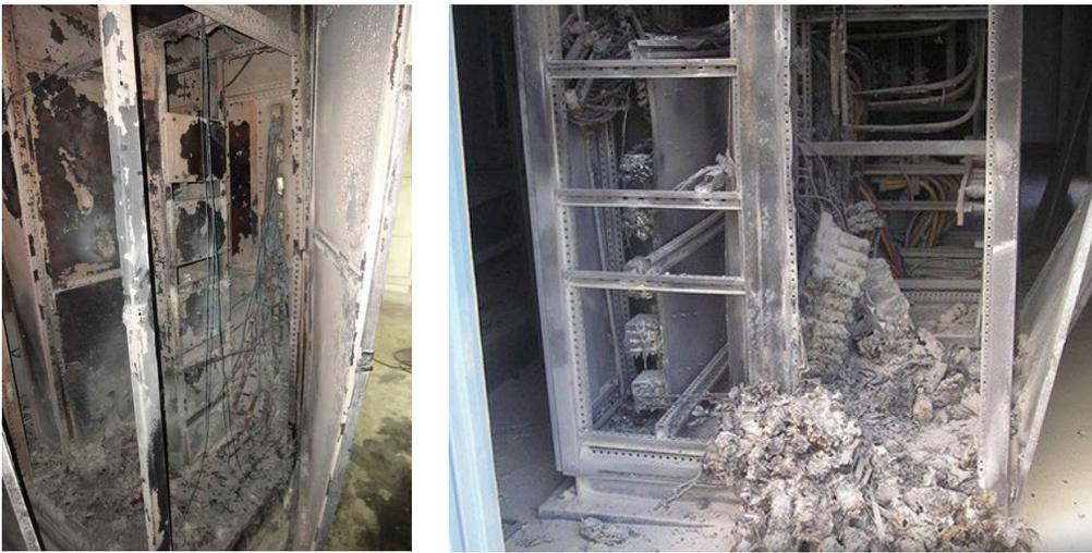
Figure 4: Catastrophic Failures of a PFC Systems – Probably Preventable with Proper CBM
