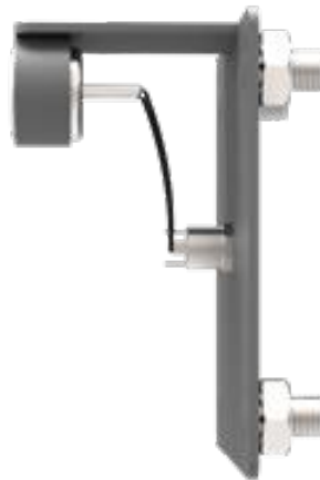
Figure 11 IR Windows with Built in Partial Discharge Sensors can be used to gather Ultrasound Data on Closed Systems
